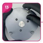
Tighten the screws of the reline jig and cure for 30 minutes at 65 °C and 2 bar pressure.
